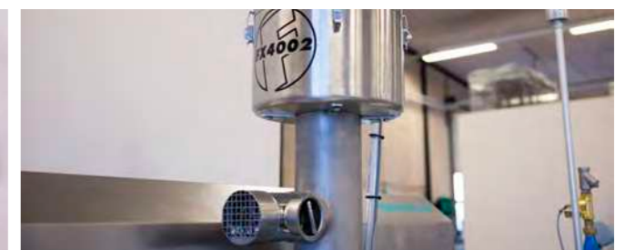
Steam condensation units
